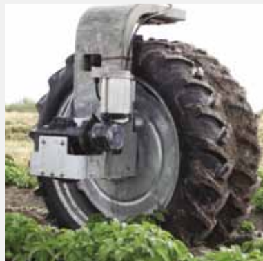
Precision Corner Dual Drive Option
