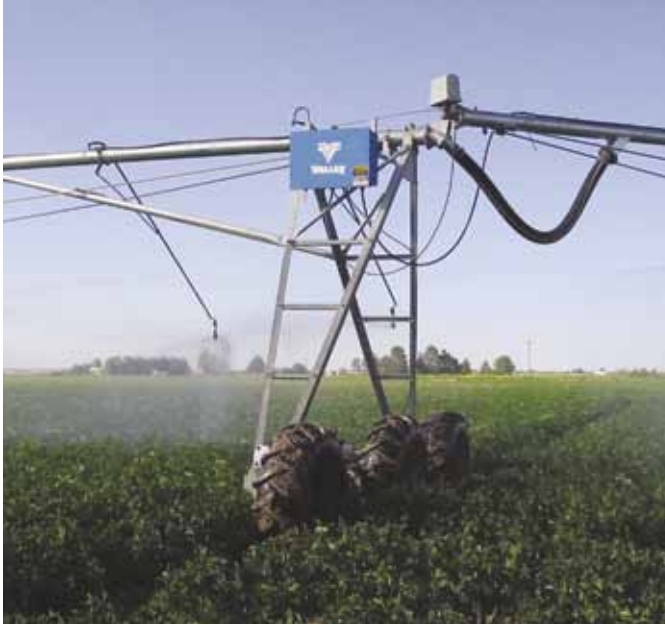
Valley, heavy duty 3-Wheel Drive option for increased traction.
