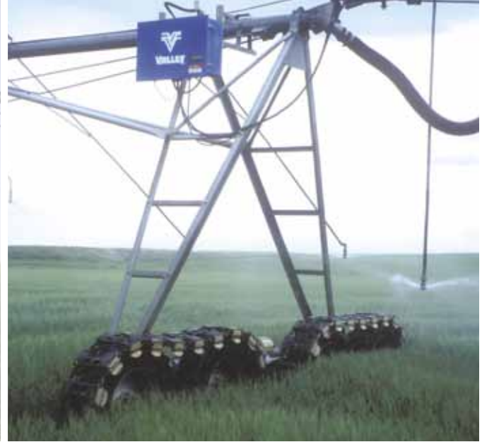
Valley, Track Drive tracked option for increased floatation.
