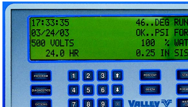
Valley Pro2 Control Panel
