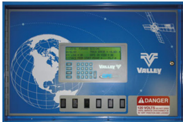
GPS Guidance Control Panel
