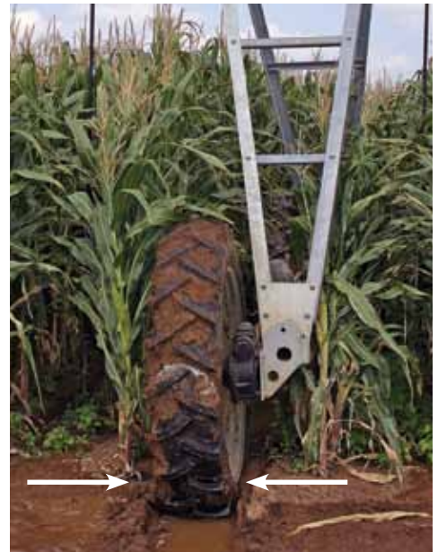
Cycle test simulates the push in and pull out loads applied to the tire, as a pivot moves around a field.
