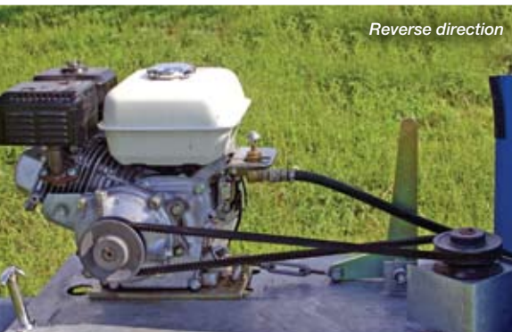
Simple over center lever is used to loosen the v-belt to reverse operating direction.
